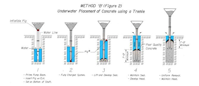
**Method B (Figure 2):** Use a tremie tube, with a pig separating the ground water and concrete, to place concrete into the shaft. Once the tremie tube is resting on the bottom of the shaft, install the pig just below the hopper in the top of the tremie tube. Fully charge the tremie tube and hopper (forcing the pig to the bottom of the tremie tube), then raise the tremie tube by 1 tremie diameter and seal the discharge end of the tremie tube with the fresh concrete.
