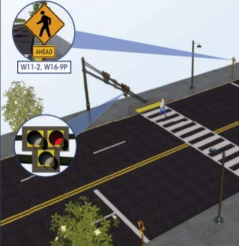
A Pedestrian Hybrid Beacon head consists of lenses above a single yellow lens. Unlike the PHB rests in dark until a pedestrian or pushbutton or other form of detection. When the beacon displays a sequence of flashing lights that indicate the pedestrian walk is safe for drivers to proceed (see figure).
