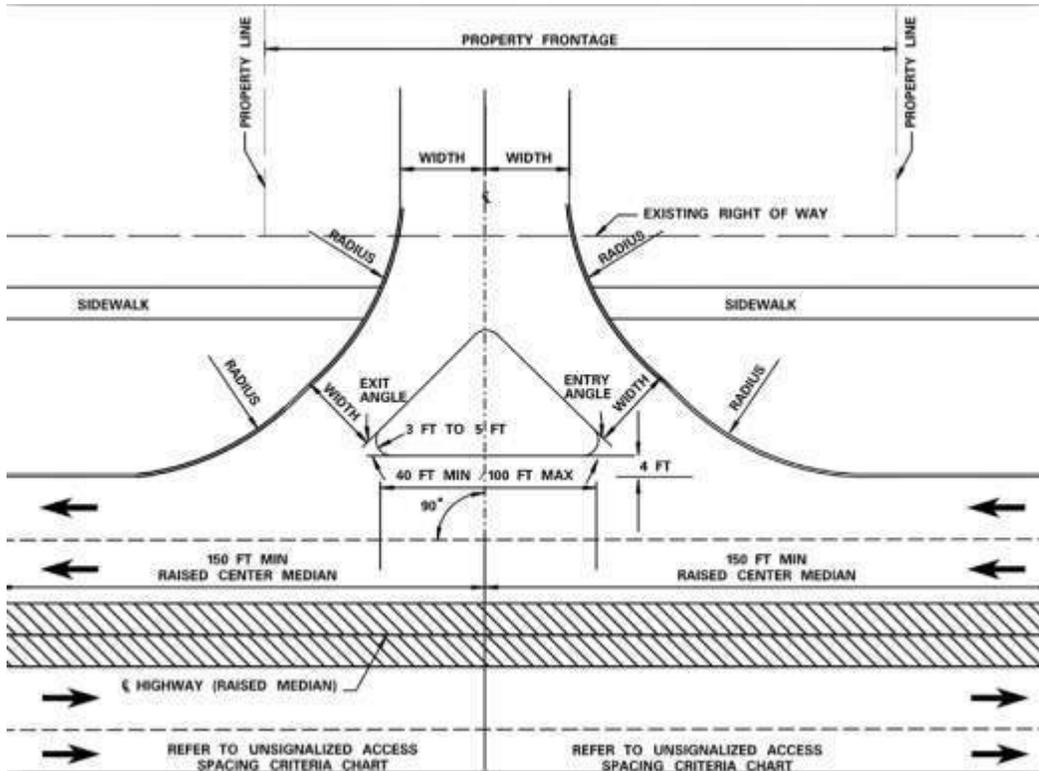
Figure 19: Right-in/Right-out Access (Source: KDOT's Access Management's Policy)
