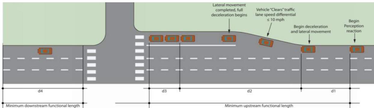
Figure 8: Intersection Functional Lengths (Source: [KDOT's Access Management Policy](#), Figure 4-17)
