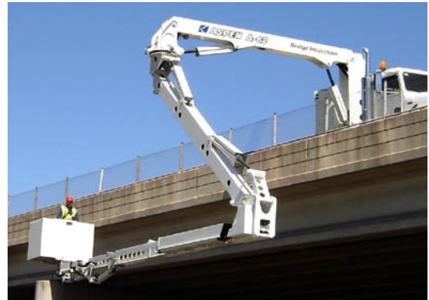
Exhibit 4.1 | Example Bridge Inspection Unit
