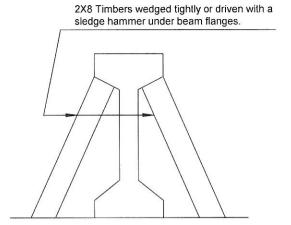
The first two beams will be set and braced like this and then the temporary steel diaphragms will be placed. After the temporary steel diaphragms are installed, move on to the next pair of beams and repeat the above process.
