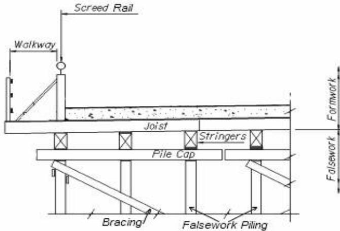
*Note: Min. vertical load to be used in the design of any falsework member shall be 100 psf measured over the total area supported by that member.*
