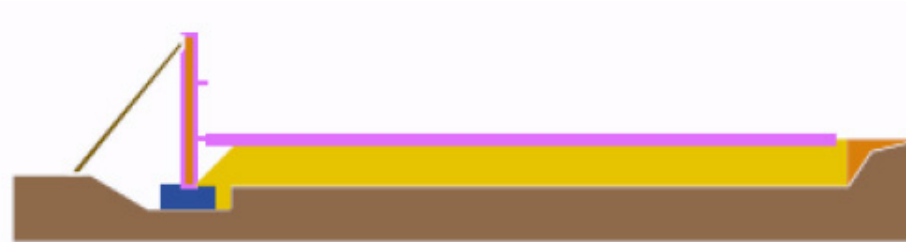
Figure 36, Connect and Tighten Reinforcement
