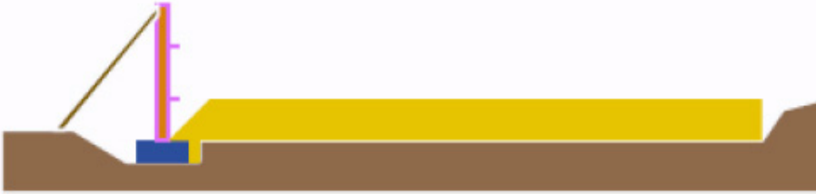
Figure 35, Fill in 10" Lifts to Reinforcement
