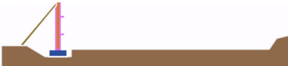
Figure 33, Install and brace first row of panels
