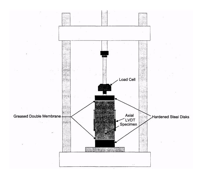
Figure 1 General Schematic of Dynamic Modulus Test
