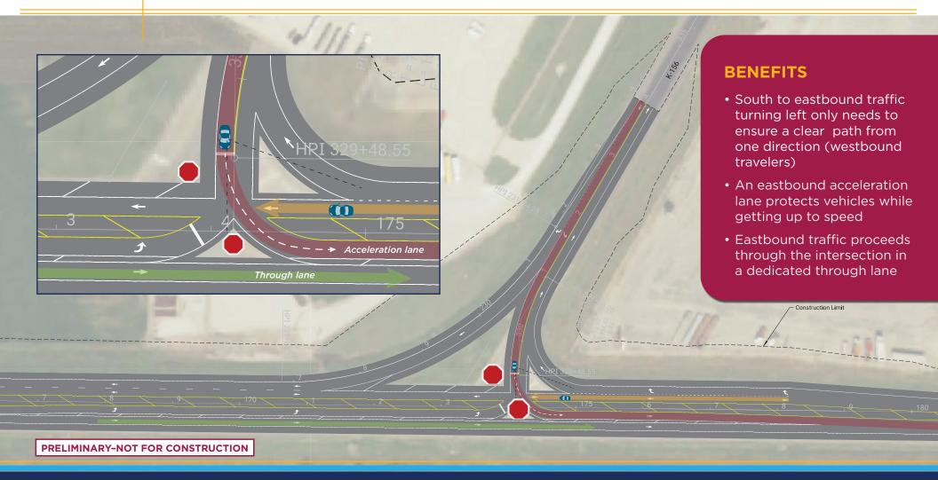
The **Continuous Unsignalized Green T** provides additional safety from a traditional T-intersection due to both the angle of the eastbound to northbound turning vehicles as well as providing a lane for the southbound to eastbound vehicles to accelerate and merge with eastbound through vehicles.
