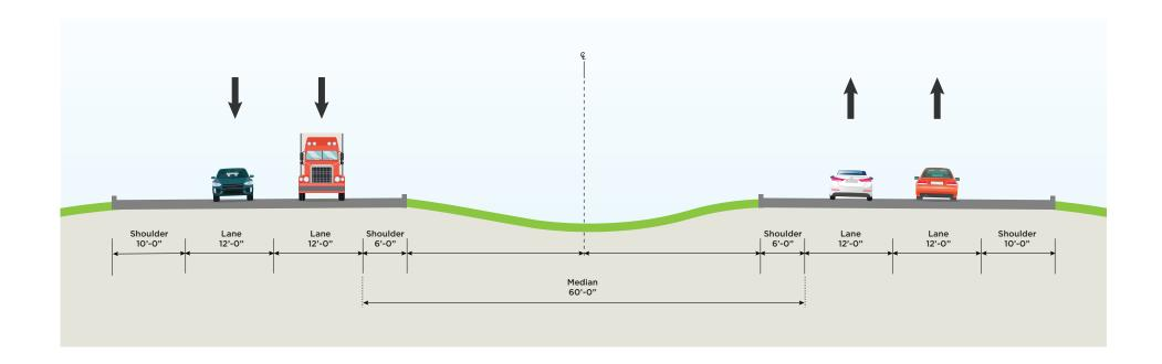
**PROPOSED 60-FOOT MEDIAN:** Typical sections are a cross section, or a driver's perspective, when looking at the roadway. The proposed improvements would include two new 12-foot travel lanes on the north. A 60-foot median includes 6-foot shoulders on the inside edge of the driving lanes, while 10-foot shoulders are proposed on the outside portion of the lanes.
