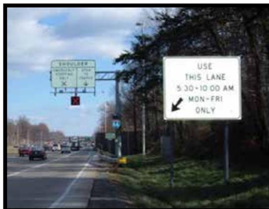
Photo of hard shoulder running on I-66 in Virginia. Shoulder running is being utilized internationally in Great Britain, Amsterdam and the Netherlands, and nationally in Washington D.C., Seattle and Minneapolis to cost-effectively manage peak hour congestion needs.
