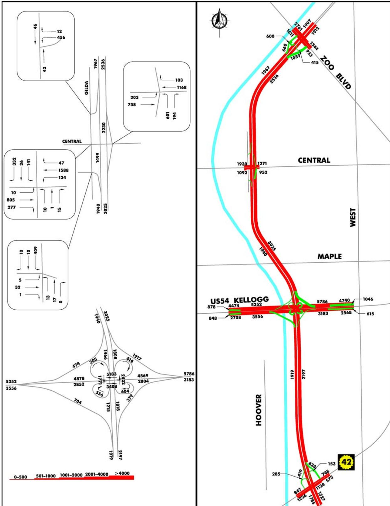
**I-235 at the junction of Central Avenue** - At this interchange, the northbound off-ramp is the most heavily traveled with nearly 800 vehicles in the peak hour. The predominant turning movement is the northbound left heading westerly. Traffic along I-235 north of this interchange is predominantly northbound (2,500/2,100 – N/S). The heaviest traffic on Central Avenue in the PM peak period is west of I-235.
